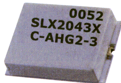
6. The SLX-2043 LNA MCM has been optimized from 1700 to 2200 MHz in order to handle a variety of wireless applications.
